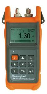
OVA-50 Optical Variable Attenuator can precisely attenuate input optical signals at 1310/1490/1550/1625nm wavelengths and directly output defined stabilized optical signals. OVA-50 is applicable in various testing situations:
